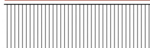
PAINTED GALVANISED STEEL BALCONY HANDRAILS
